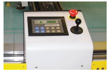
The easy-to-use keypad controls multiple machine functions at the cutter.
